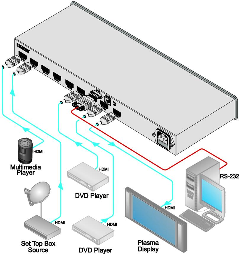
Figure 2: Connecting a VS-81H 8x1 HDMI Switcher
