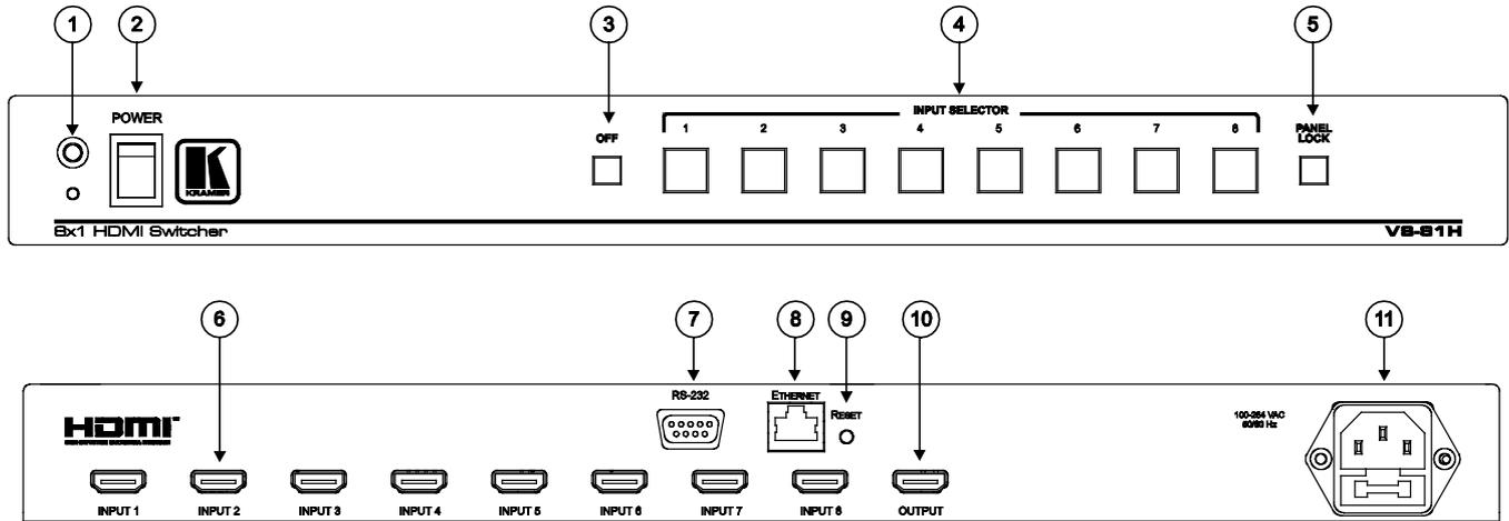
Figure 1: VS-81H 8x1 HDMI Switcher
