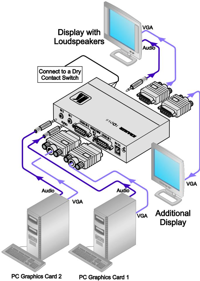
Figure 2: VP-211K Automatic UXGA / Audio Switcher Connections
