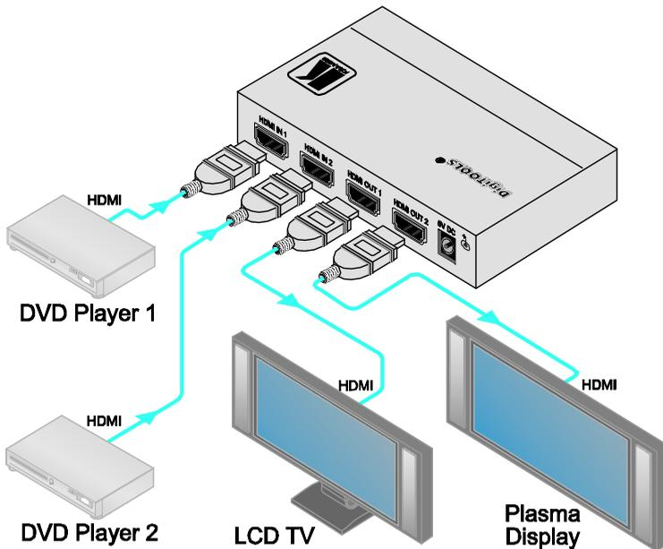
Figure 2: Connecting a VM-22H 2x1:2 HDMI Switcher/DA
