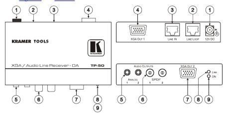
Figure 1: TP-50 XGA/Audio Line Receiver - DA
