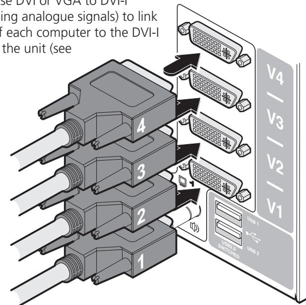
*Note:* On the rear panel of the unit, connectors belonging to the same channel are stacked vertically. The connectors at each horizontal level (V1 to V4) will be switched through to the user console DVI-I connector which is at the same level:
