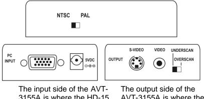
3155A is where the HD-15 PC input connector and the 5VDC Power adapter connectors are located. The output side of the AVT-3155A is where the S-Video, Composite Video connectors and the Overscan/Underscan switch are located.
