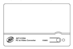
The Power Switch and Power "On" LED are located on the top of the unit. The NTSC/PAL switch on the front of the AVT-3155A allows selection of the desired television standard.
