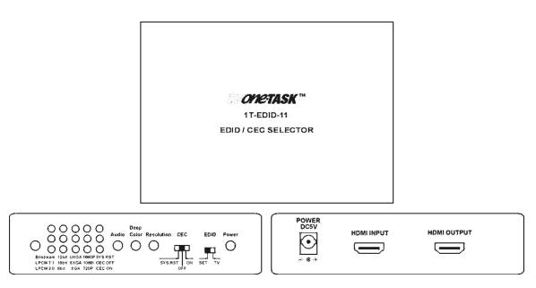
Connect the source device's output to the HDMI IN connector of the 1T-EDID-11 using a high quality cable.
