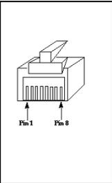
The diagram shows a top-down view of an RJ45 connector. It has eight pins arranged in two rows of four. The top row is labeled 'Pin 1' and the bottom row is labeled 'Pin 8'.
