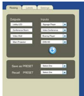
Figure 13 – Typical Web Control
