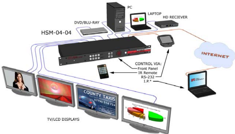
Figure 6 – Connection Block Diagram
