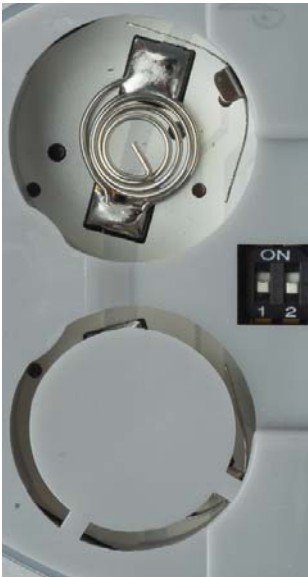
Left: Picture of the opened rear battery compartment of the RMT-2IR remote showing the exposed DIP Switch bank between the battery chambers.
