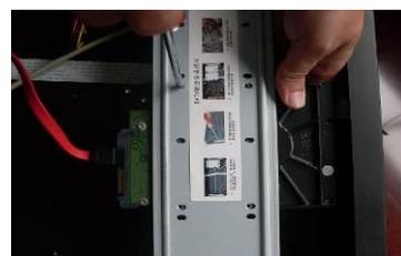
3. Use four screws to fix HDD.
