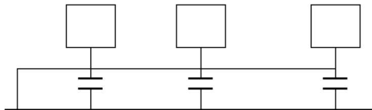
When connecting devices of huge size (the device physical dimension and connection cable is big comparing with the wave path of existed interference), then there are possibilities of interference when the current goes through the chassis and cable. In this situation, the interference circuit path usually lies in the system ground circuit.
