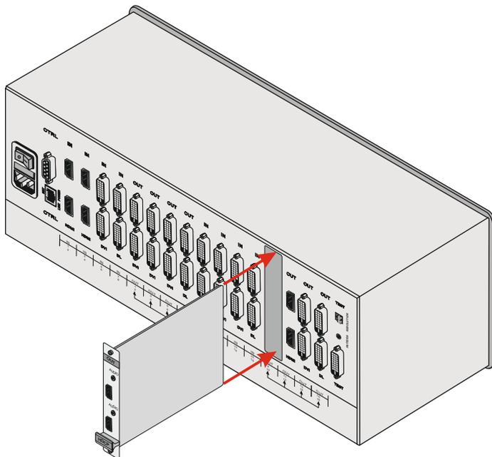
5. Holding the card by the upper handle, align the card with the plastic guide rails.
