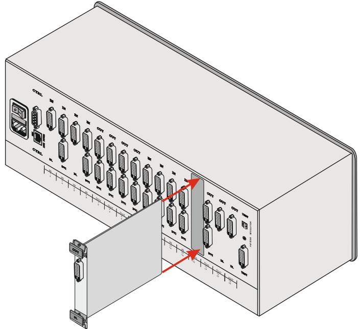
5. Holding the card by the upper and lower handle, align the card with the plastic guide rails.
