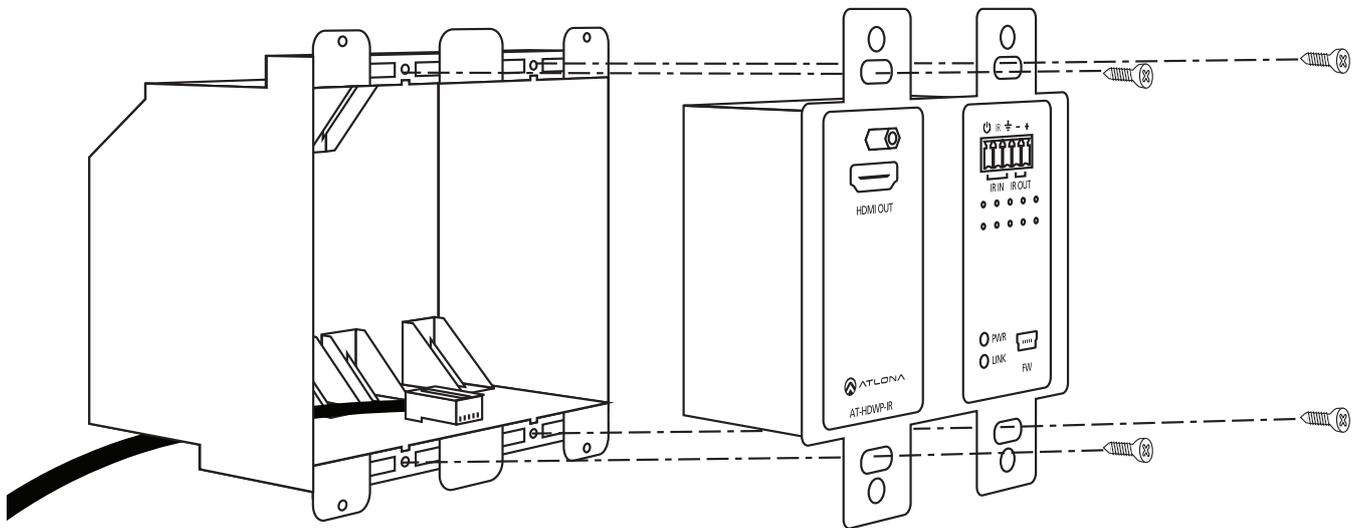
The first step in installation is to connect the cat cable to the Decora HDBaseT module and install it into the electrical box (as seen above).
