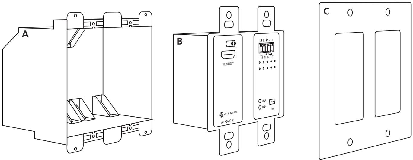
There are four pieces that will need to be interconnected in order for the AT-HDWP / AT-HDWP-IR to be installed in the wall. The electrical box (picture A), the Decora HDBaseT module (picture B), the Decora face plate (picture C) and the CAT cable.
