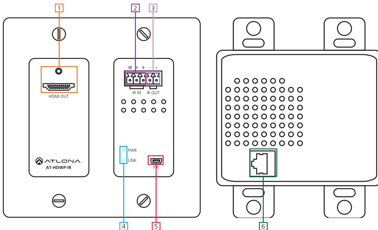
1. HDMI OUT Port: Connect to HDMI display.
