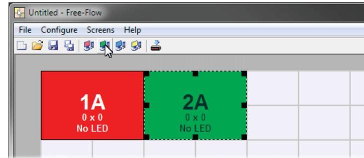
*Note: By default, the Free-Flow screen will automatically add four screens in a straight row (1A 2A 3A 4A), each at a resolution of 1920 x 1080. You can edit or delete these screens as required.*
