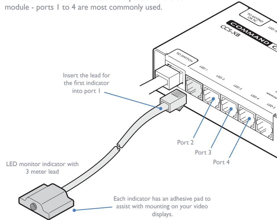
3 You need to tell the CCS-PRO4 which LED monitor indicator to illuminate (and in which colour) for each channel. To do this connect your computer to the CCS-PRO4 switch via a [network connection](#) and use the Free-Flow application. Please see the section [Configuring LED monitor indicators](#).
