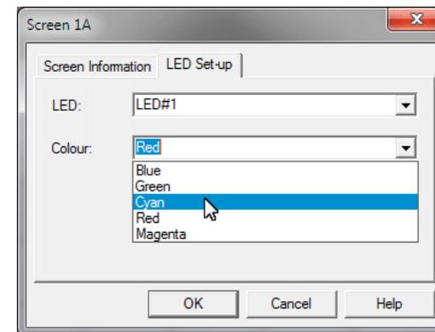
*Note: Each LED indicator can only have one colour, so if you associate an indicator with more than one screen and then change the colour on a later screen assignment, it will be changed for all the screens in the list for that LED indicator.*
