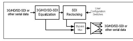
The DA-3G-1x6 can be operated in automatic standard detect mode or in a manual standard mode. Reclocking can be bypassed if desired. Non-inverting ASI reclock is available on 3 of the 6 output ports.
