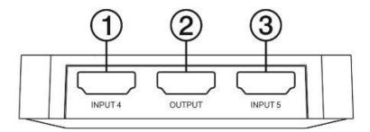
$\underline{\rm Rear \ Panel:} (1) (2) (3)$  HDMI input ports, connect with Blu-ray Player, PS4, Cable Box, Laptop, and Xbox One with HDMI cables
