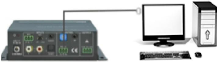
**Figure 10 Connection of RS232 Port**
