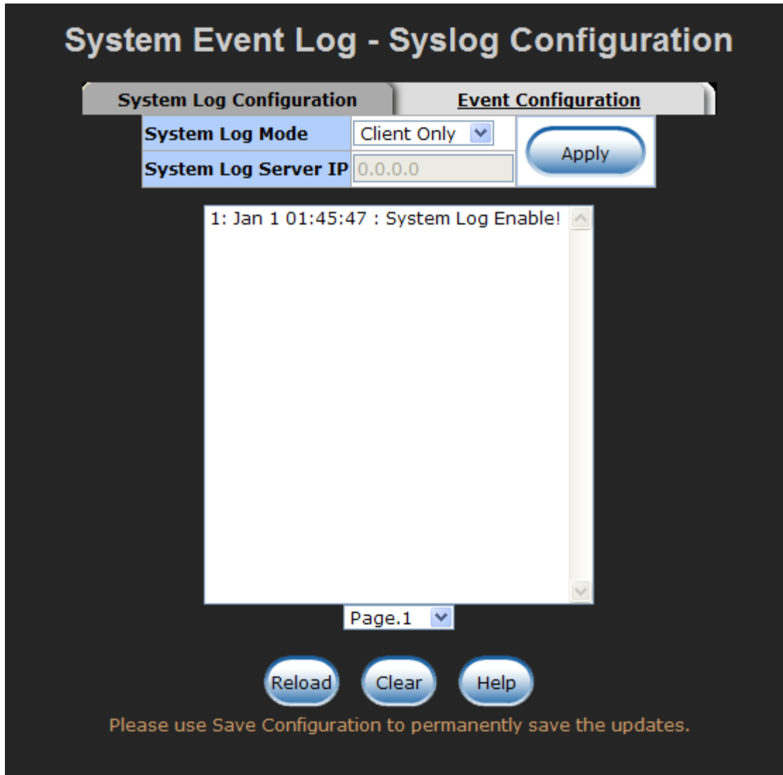
System Log Configuration interface
