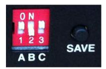
Turn OFF switch 2, then press SAVE to reset the display EDID data.
