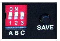
Turn ON switch 2. Select settings for switch 3, then press SAVE to store internal EDID data.
