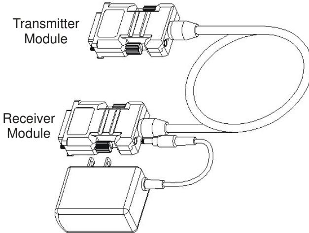
*Figure 1: Optical DVI Extension Cable*
