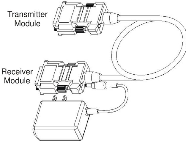
*Figure 1: Optical DVI Extension Cable*
