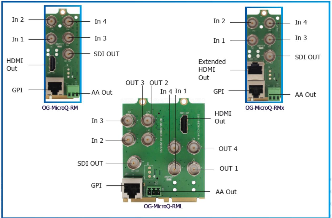
Figure 1: OG-MicroQ Rear Module
