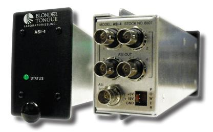
The ASI-4 is a 1:4 active ASI splitter. It is designed to complement digital headend products that can utilize an ASI input for EAS (Emergency Alert System) applications, or any application requiring splitting of an ASI signal. The ASI-4 can be deployed in a daisy-chain configuration to provide additional outputs as required. Modular design allows installation of up to six units in 2RU.
