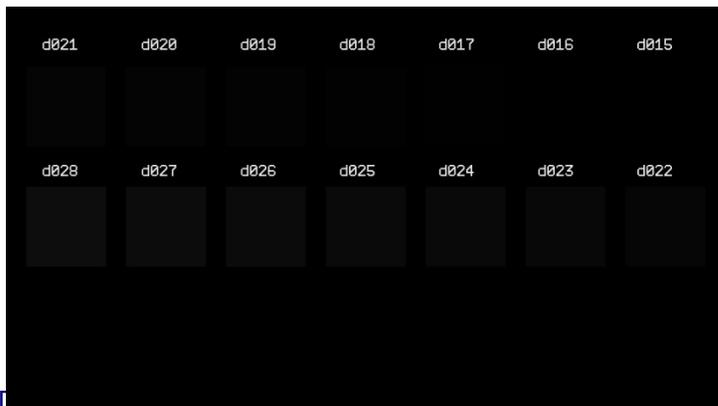
RGB video is normally sent using all 256 bits (in 8 bit color) but YCbCr (component video) sets black at 16 and white at 238. This allows room above and below the active video for below black and above white. PLUGE patterns are specifically designed to allow quick visual setting of the black and white level.
