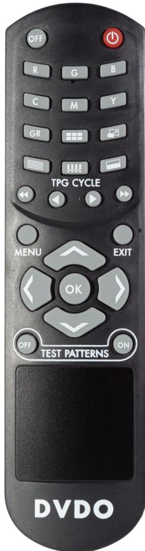
The AVLab TPG remote is specifically designed to allow fast access to patterns. Choose a pattern category using the top bank of buttons, then use the cycle buttons < and > to choose different patterns within that category. << and >> changes between categories.
