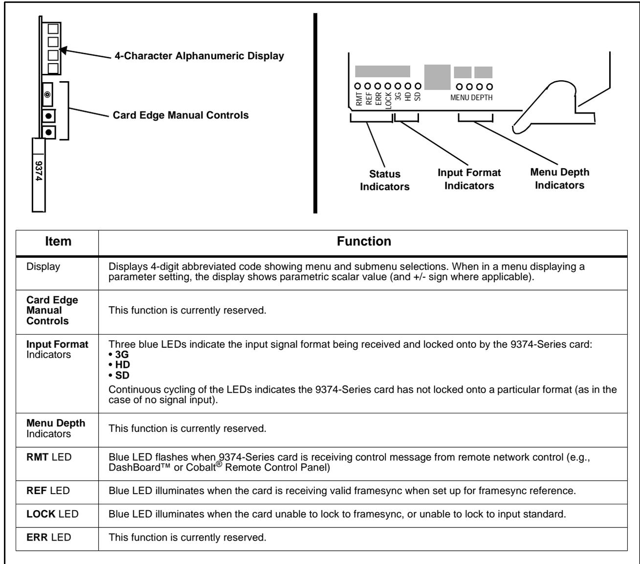
**Figure 3-2 9374-Series Card Edge Controls, Indicators, and Display**
