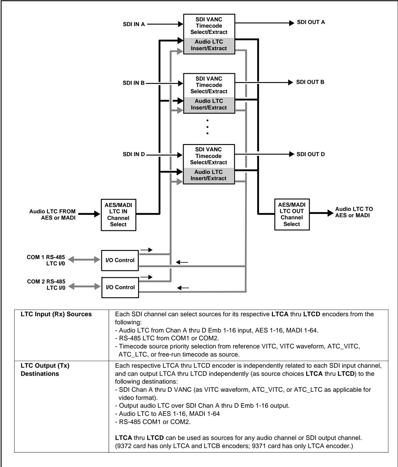
Figure 1-3 Timecode Interfaces Using Option +LTC
