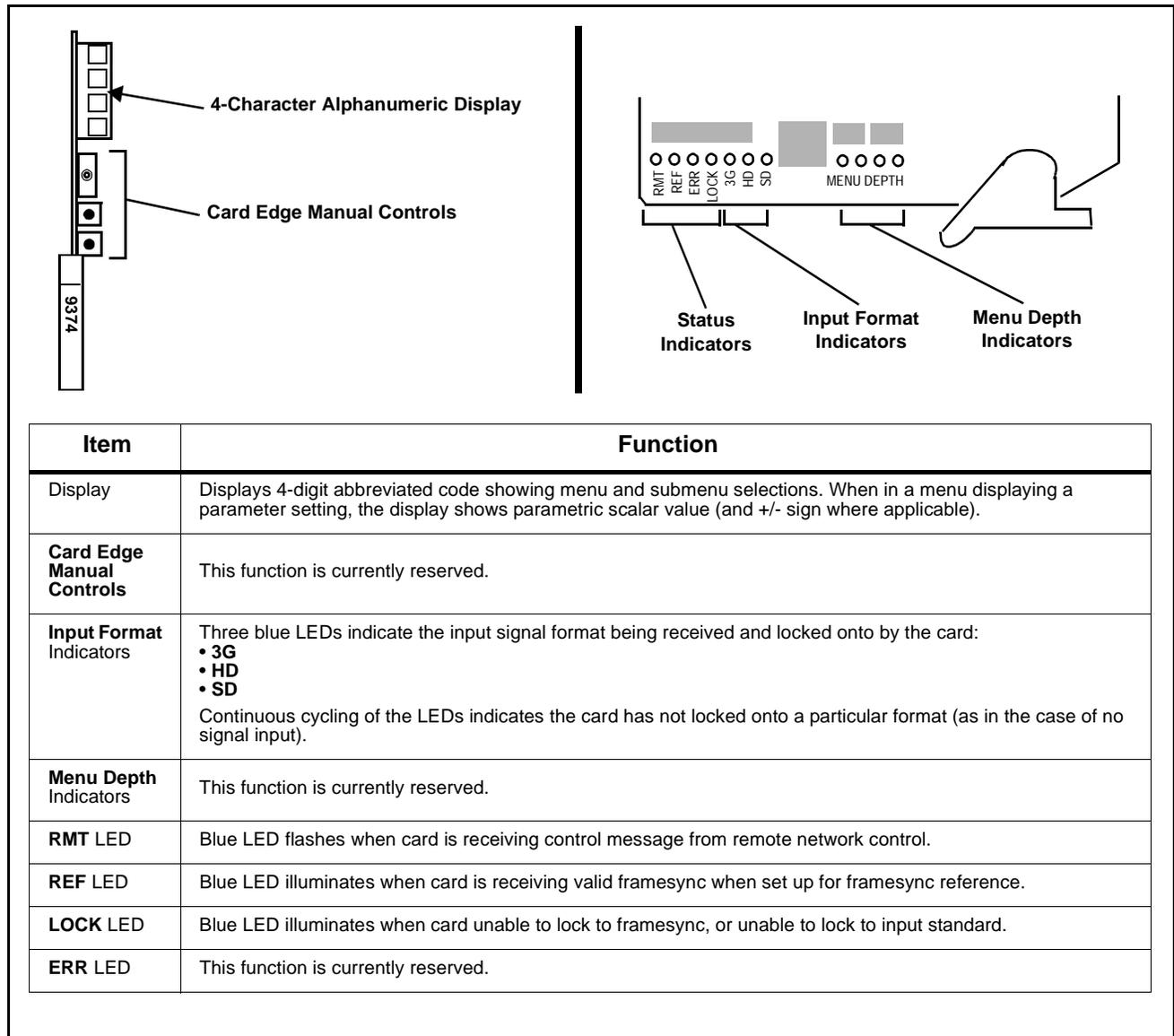
Figure 3-5 9374-Series Card Edge Status Indicators and Display
