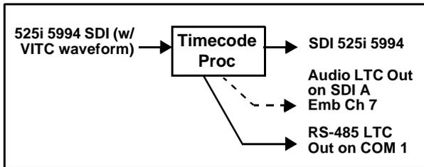
Noting that program material VITC waveform timecode is only to be used, **Source Priority 1** is set to prioritize SDI VITC as the only choice. Therefore, when VITC waveform is present, it will be considered as the source that will eventually be outputted by the card regardless of output format selected.
