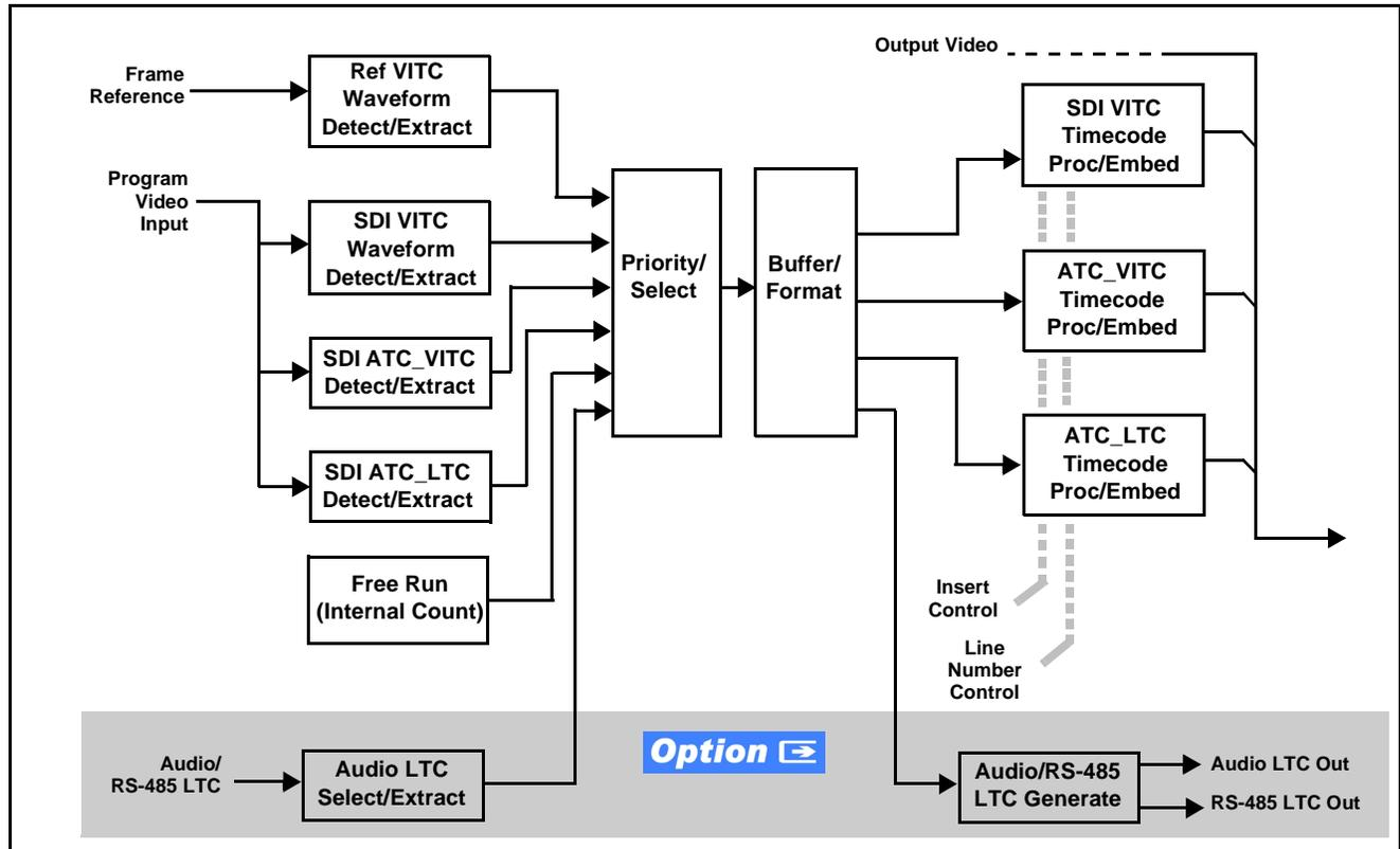
Figure 1-2 Timecode Processor (One Channel Shown)
