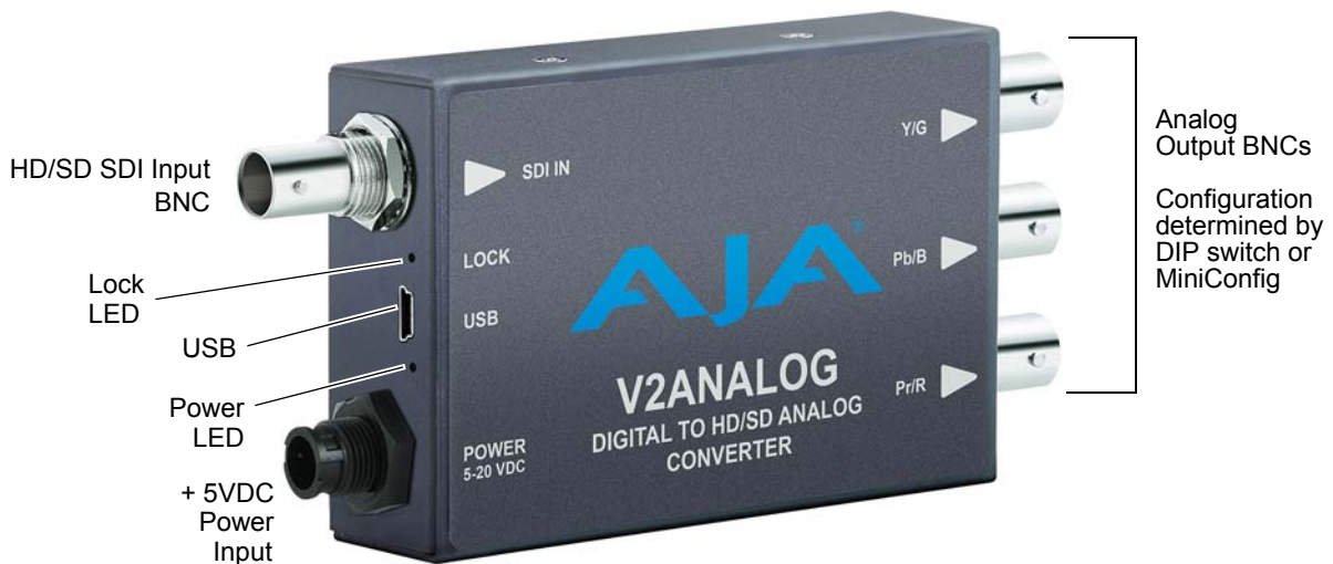
Figure 2. V2Analog I/O Connectors
