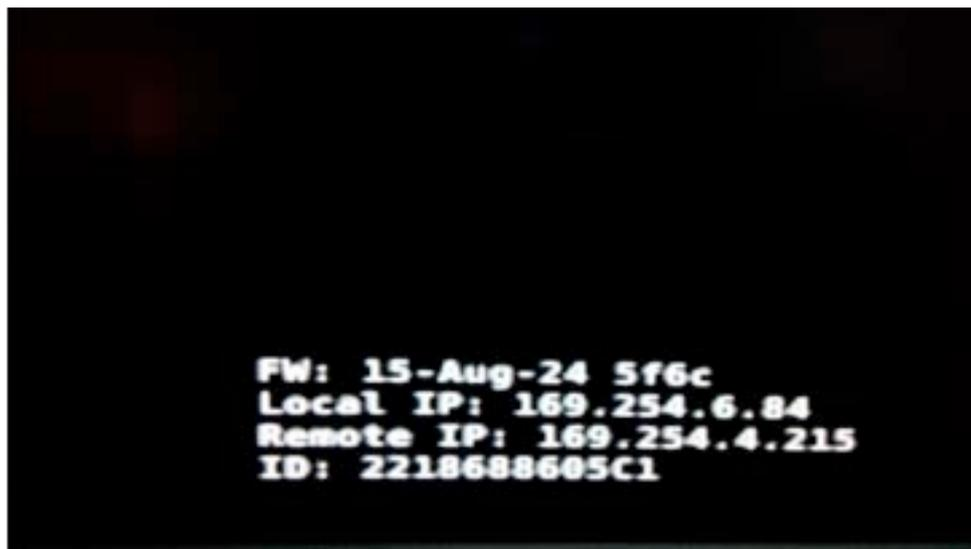
Fig. 6-10: Initial OSD Screen capture when KVM-1-RH-LAN is connected to the screen without any network
