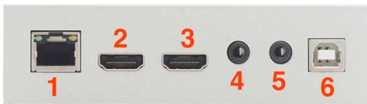
Figure 6-1: Connect the USB cable between the source computer to KVM-1-EH-LAN via port 6
