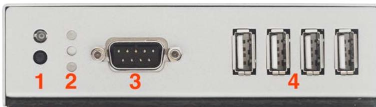
Figure 6-2: Connect the physical mouse and keyboard to the USB ports marked as "4"
