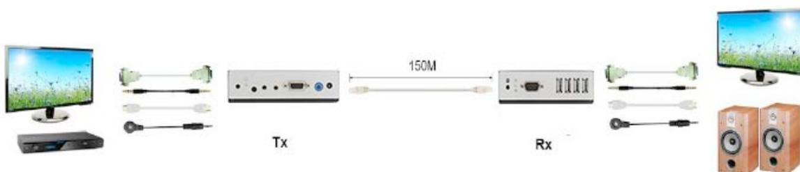
Figure 6-4: Point to point connection
