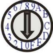
This KVM system is capable of 16 transmitters to 200 receivers. This rotary switch has 16 positions to enable the required channel settings.
