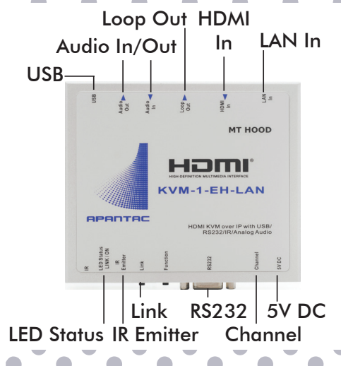
KVM-1-EH-LAN Single-port HDMI/USB/RS232/IR KVM Extender over Ethernet
