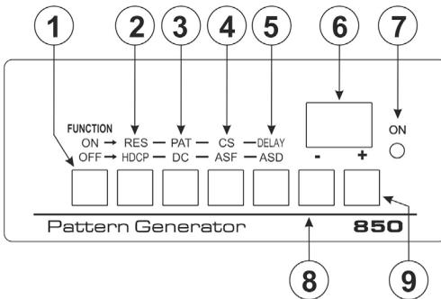
Figure 1: 850 Pattern Generator Front Panel
