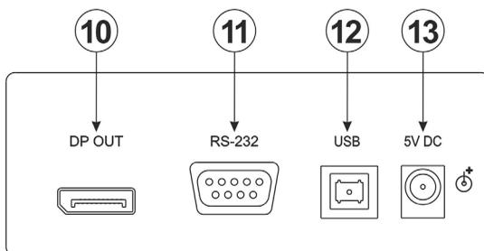
Figure 2: 850 Pattern Generator Rear Panel
