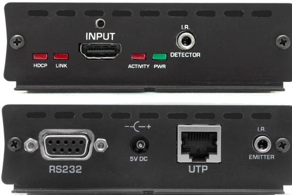
Figure 3 - Sender Connections (UHBX-S-PSE shown above)
