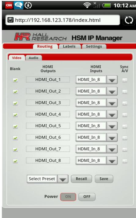
Figure 11 – Video routing sub tab
