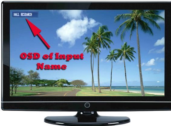
Figure 6 – On Screen Display of user defined input names after switching (position and duration is configurable)
