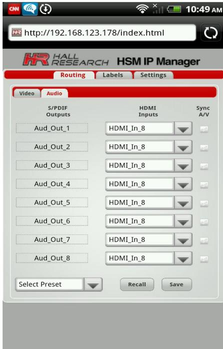
Figure 12 – Audio routing sub tab
