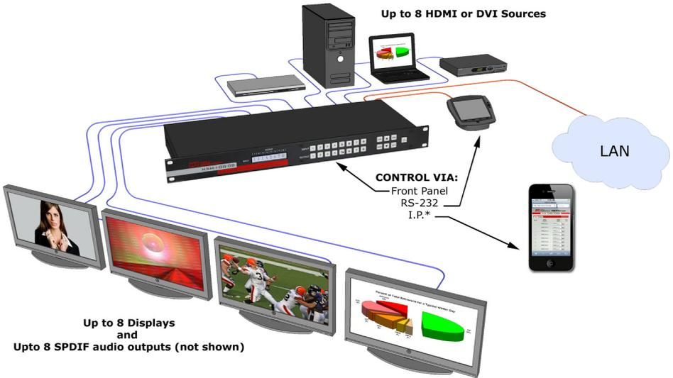
Figure 5 – Connection Block Diagram
