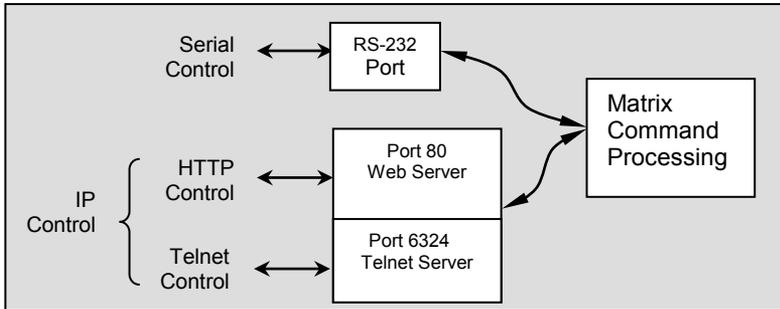
Figure 8 – IP Control Block Diagram
