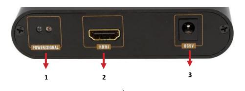
1: LED Indicator: Power LED when powered GREEN / Signal LED when signal is transmitting RED
