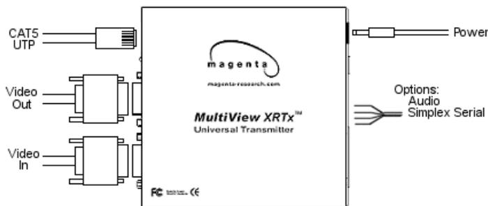
**Figure 3-1. Connections on the XRTx Universal Transmitter.**
