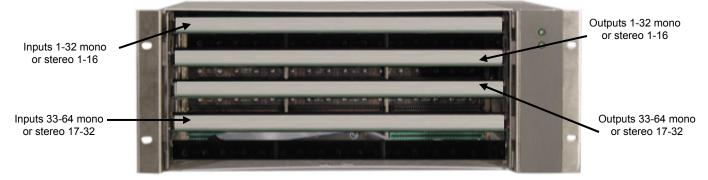
The top slot in both the analog and digital frame contains the input buffer module for inputs 1-32. The next  $(2^{nd})$  slot down contains the crosspoint/output driver module for outputs 1-32. The  $3^{rd}$  slot from the top contains another crosspoint/output driver module for the outputs 33-64. The  $4^{th}$  slot from the top contains an input buffer module for inputs 33-64.
