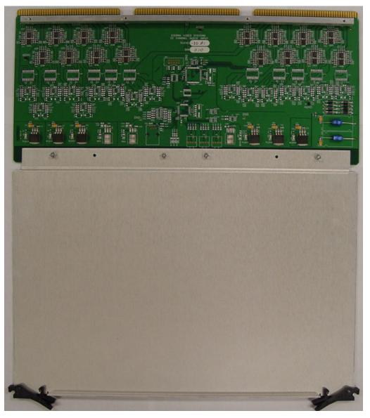
The output of the input buffer circuits are connected to the switching matrix via the internal motherboard. Unlike their analog video counterparts, the input buffers are internally mounted. The 64x64 frame has positions for two 32-channel buffer modules; and the 128x128 frame has positions for four 32-channel buffer modules.
