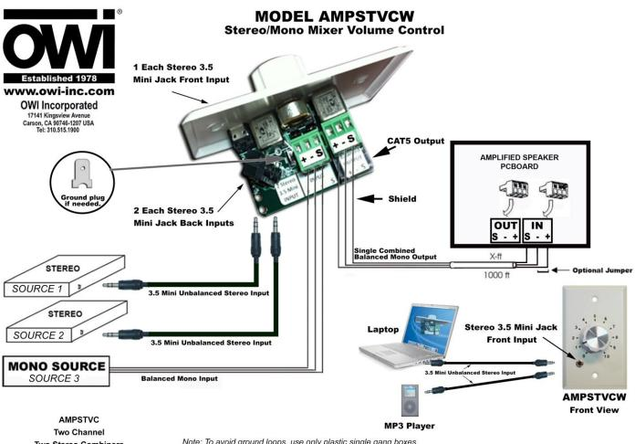
Two Stereo Combiners Takes Stereo Converts to Mono **Transformer Balanced**
