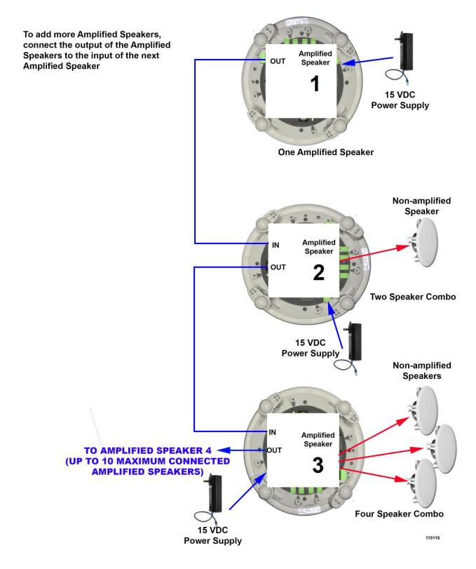
**One, Two, Four Speaker Combination Wiring**
