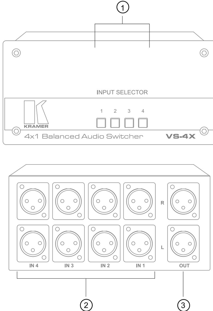
**Figure 3: VS-4X Front/Rear Panel Features**
