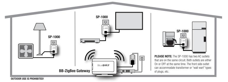
Multiple SP-1000 units can be installed within 100 ft. from an active ZigBee device (BB-ZIGBEE Gateway, MD2-ZB or another SP-1000).
