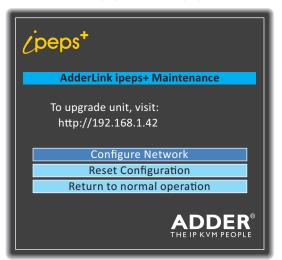
Note: When an AdderLink ipeps+ unit is put into recovery mode, if the Configure Network option is then used to change the IP address, this change will only apply whilst the unit remains in recovery mode. Once recovery mode is exited, the unit will revert to the previous IP address.
