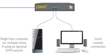
The AdderLink ipeps+ module is contained within slimline metal casing measuring just 169 x 112 x 31mm.
