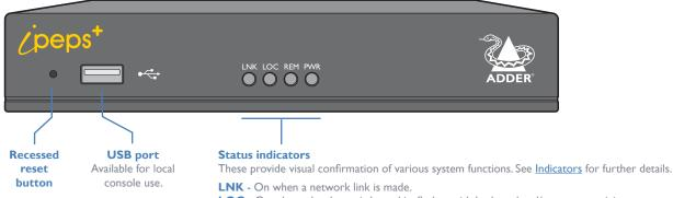
LOC - On when a local user is logged in, flashes with keyboard and/or mouse activity. **REM** - On when a remote VNC user is logged in, flashes with keyboard and/or mouse activity. PWR - On blue when power is present, flashing red when upgrading or in recovery mode.
