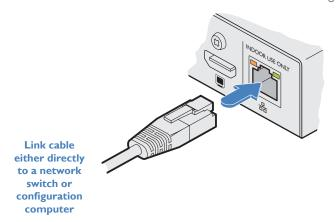
2 Connect the other end of the cable either directly to a suitable network switch.
