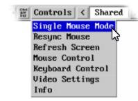
To quit from single mouse mode, press F8 and then P.Alternatively, enable and use the mouse button escape sequences - see Advanced unit configuration for details.
