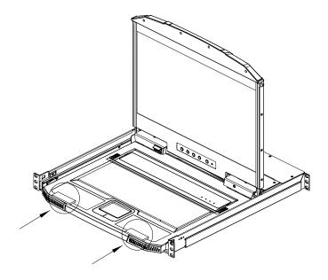
4. The LCD KVM switch is designed for rack mounting. If the KVM switch is not rack mounted be sure to place it on a completely flat and firm surface before pulling the device in or out to prevent damage due to uneven force on the module.
