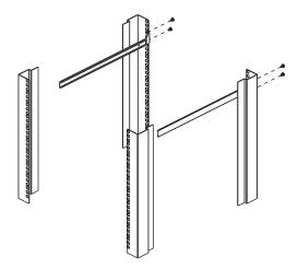
2. While one person inserts the CL3800 / CL3700 / CL3100 into place by sliding its left and right side bars into the mounting brackets (on the rack), have a second person install four screws in the front tabs to secure the module to the front of the rack.
