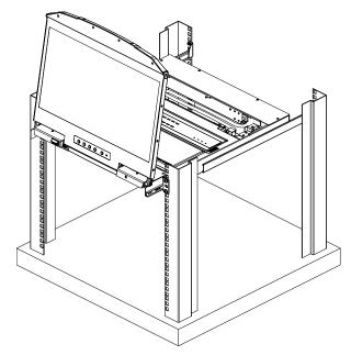
7. To close the LCD screen, lower the panel module until it lies flat and slide it back in.
