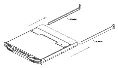
2. Attach the left and right *easy-installation* mounting rails to the inside of the rack. The flange that supports the CL3800 / CL3700 / CL3100 will be to the inside.
