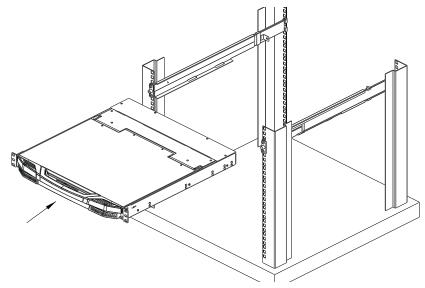
4. Slide the rear attachment sliding brackets along the slide bars until they contact the rear of the CL3800 / CL3700 / CL3100, then use the screws supplied with this package to attach the bars to the rear of the CL3800 / CL3700 / CL3100 (tighten the screws all the way).
