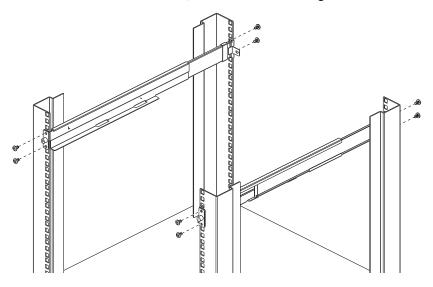
3. Slide the CL3800 / CL3700 / CL3100 onto the support flanges. Use the screws supplied with this package to loosely attach the front of the CL3800 / CL3700 / CL3100 to the front of the rack (only tighten the screws part way).
