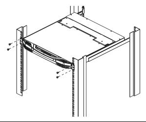
**Note:** Allow at least 5.1 cm on each side for proper ventilation, and at least 12.7 cm at the back for the power cord and cable clearance.
