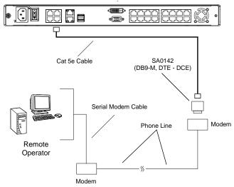
2. From your client computer, use your modem dial-in program to dial into the KN1108VA / KN1116VA modem.
