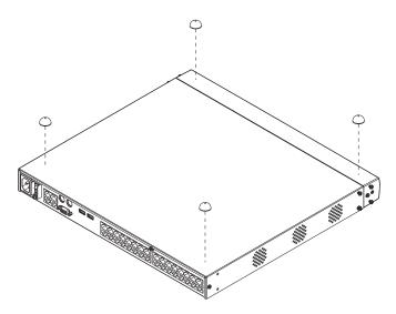
**Note:** To ensure adequate ventilation, allow at least 5.1 cm on each side, and 12.7 cm behind the unit for power cord and cable clearance.
