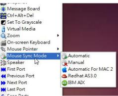
• Linux doesn't support DynaSync Mode, but there is a setting on the Mouse Sync Mode menu for Redhat AS3.0 systems. If you are using a USB Adapter Cable (see the Note on the previous page), with an AS3.0 system and the default mouse synchronization is not satisfactory, you can try the Redhat AS3.0 setting. In either case, you must perform the manual mouse synchronization procedures described in the next section.
