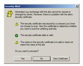
The certificate can be trusted, but the alert is triggered because the certificate's name is not found on Microsoft's list of Trusted Authorities. You have two options: 1) you can ignore the warning and click **Yes** to go on; or 2) you can install the certificate and have it be recognized as trusted.
