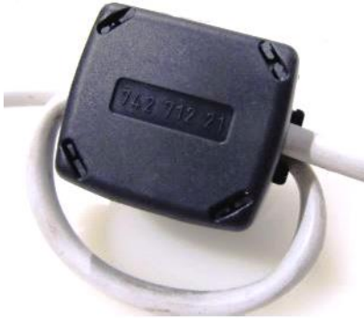
Figure 6: Looping the Cable through the Ferrite Ring
