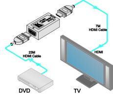
The **PT-2H** input is connected via a long male-to-male HDMI cable (not provided) to an HDMI source, such as a DVD player or a satellite set top box.
