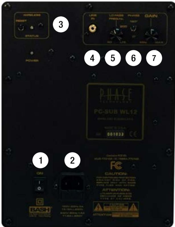
1. Power/Auto ON/OFF: When this switch is left “ON”, the subwoofer automatically activates upon detection of an audio signal; the subwoofer goes into “STANDBY” after approximately ten (10) minutes of silence. The LED on the amplifier will change from Red to Green when an input signal is detected and the amplifier turns on.
