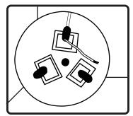
2. Locate speaker wire on the underside of the speaker. Strip wire ends if neccessary.
