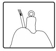
2. Locate speaker wire on the top of the speaker. Strip wire ends if neccessary.
