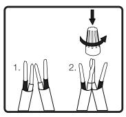
3. Connect the speaker wire to the input signal wire. Red is positive, black is negative.
