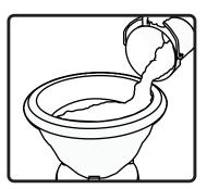
4. Place speaker in desired location. Fill planter with pea-gravel to approximately 2" above the black insert box to ensure proper drainage. Gently rock the planter from side to side so that gravel fills in the gaps, providing ample coverage of interior black speaker box.
