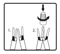
3. Connect the speaker wire to the input signal wire. Red is position, black is negative.
