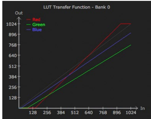
Figure 36. Example LUT Transfer Function Curves
