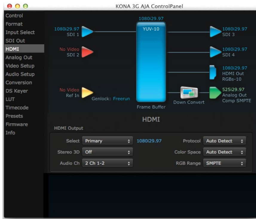
Figure 23. AJA Control Panel, HDMI Screen
