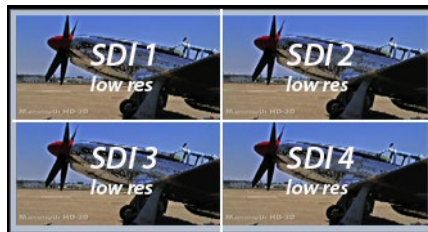
Figure 42. Mapping of 2SI Outputs
