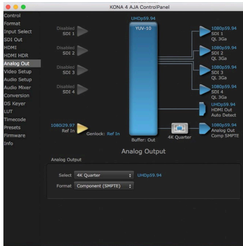
Figure 49. AJA Control Panel, Analog Out Screen with 4K Primary Format
