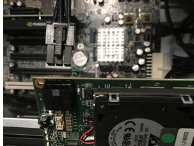
Figure 9. KONA 5 ATX Power Connection
