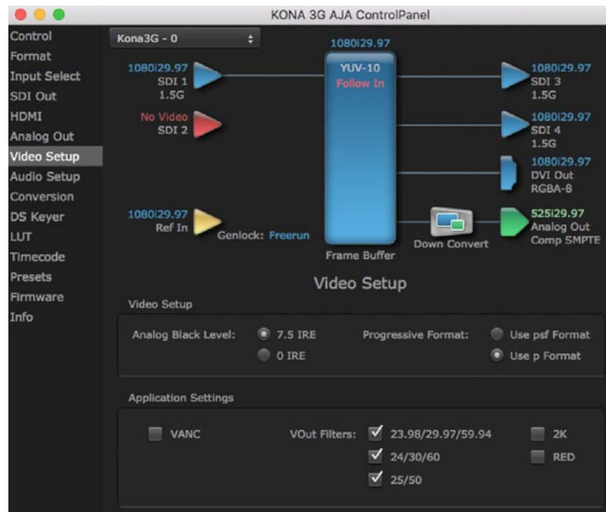
Figure 25. AJA Control Panel, Video Setup Screen
