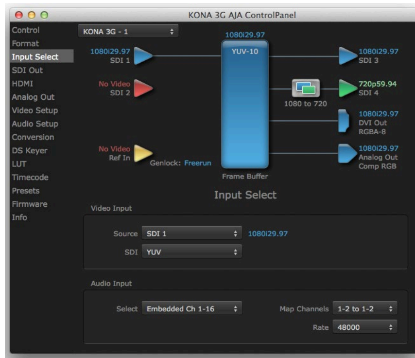
Figure 21. AJA Control Panel, Input Select Screen
