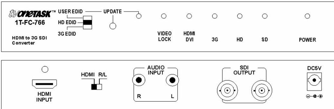
Connect the HDMI source device's output to the HDMI IN connector of the 1T-FC-766, using an appropriate high quality HDMI cable.
