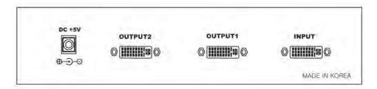
DC +5V: Power Receptacle INPUT: DVI –D connector OUTPUT1, 2: DVI Output
