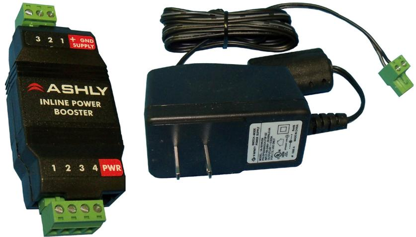
Ashly offers the RPS-18 Inline Power Booster for a 100-240V, 50-60Hz AC adapter providing 24VDC and 625mA maximum current. It uses euroblock terminals on both ends for easy insertion between the host unit's Remote Data Connection and WR-5 Input jack as shown below:
