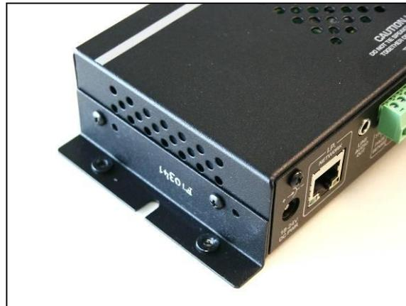
Bracket installation for surface mounting
