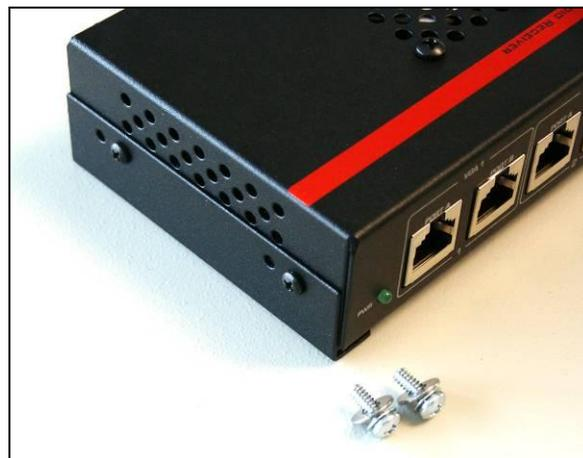
Bracket installation for vault mounting
