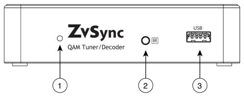
① LED Status Indicator – Indicates state of unit. *RED* – Power is available, but unit is DEACTIVATED *GREEN* – Unit is powered-up and ACTIVATED
