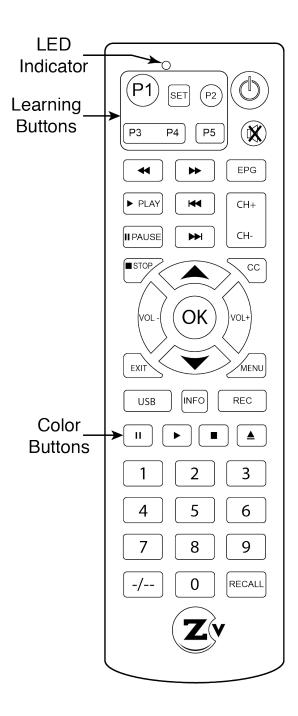
The ZvSync receiver/decoder is supplied with a partial learning remote control device. Buttons P1-P5 can be programmed to mimic the functions of a select set of buttons from another remote control unit.
