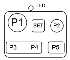
The upper-left portion of the remote houses a set of programmable keys. The intent is to allow for common television functions to be programmed so the user only needs to use a single remote control device to manage their television experience when using the ZvSync receiver/decoder.
